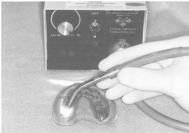
FIG. 2—TRIAD resin gel (Dentsply International, York, PA) in impression being cured using portable visible light curing unit.
