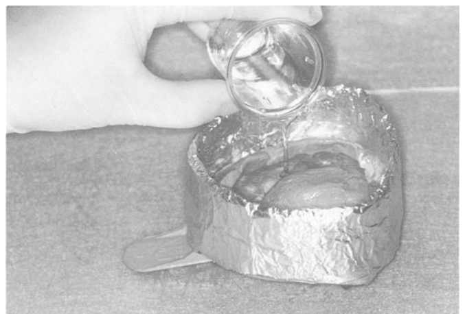
FIG. 4—Upper impression boxed using wax and aluminum foil. Marglass 658 epoxy resin (Acme Chemicals and Insulation Co., New Haven, CT) is poured into the impression and allowed to cure with the impression being maintained in a horizontal and level position.
